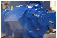
The JS solution also provided a more continuous flow, lower pressure and less wear on the pipeline. The JS Lamella Pump is significantly less noisy and takes up little space compared to the piston pump.
