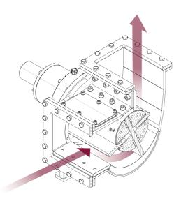
The rotor is suspended eccentrically in the pump house. Two lamellas are placed in the rotor which creates four large pumping chambers. The lamellas are guided by the cam discs in the pump housing, thereby causing a displacement of the product.
