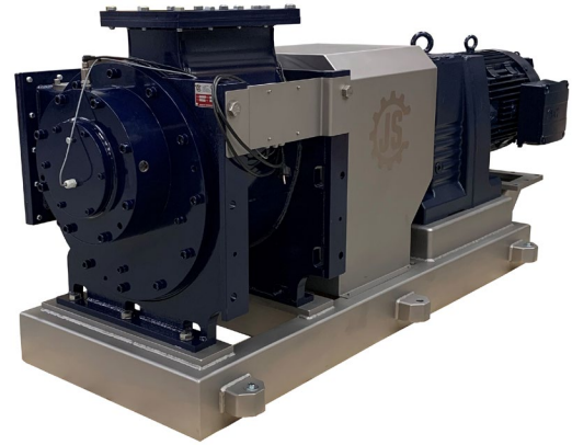
The JS Maintenance Mate box mounted on a JS Lamella pump.
